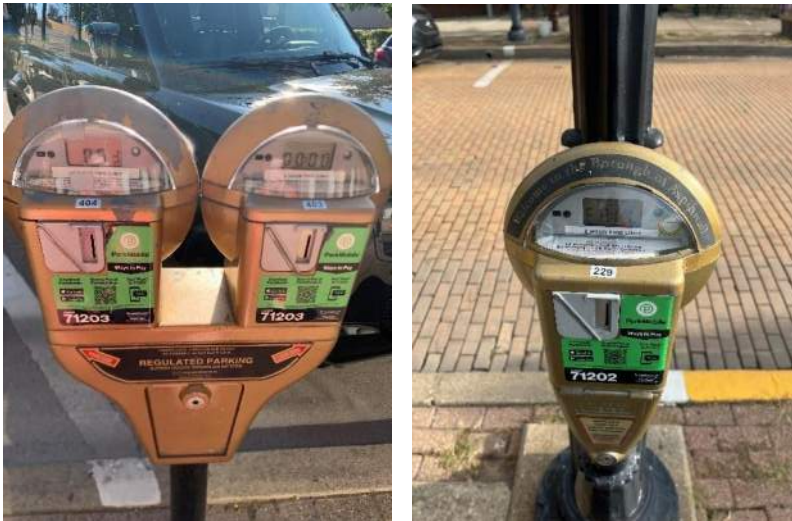
Figure 12: Single Space Parking Meter
