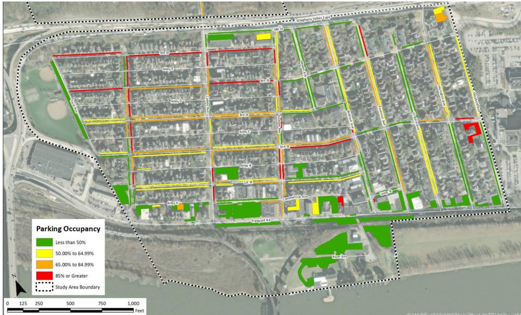
Figure 27: Lower Aspinwall 8:00 pm Parking Occupancy
